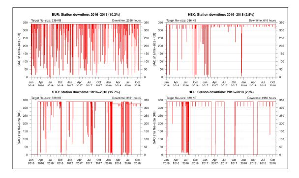
Figure 12. Downtime for the strainmeter stations for the period 01.01.2016–01.11.2018 expressed as completeness of the daily SAC file size. A complete file is represented by a horizontal flat red line with a file size of 339 KB, whereas missing data are represented by the vertical red lines.
