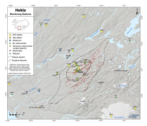
Figure 7. Overview of the current monitoring network of Hekla volcano.
