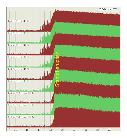
Figure 6. Tremor plot (scaled RSAM) displaying averaged seismic amplitude data (in different frequency bands) from the seismic station HAU. The yellow line represents the onset of the eruption. The horizontal axis displays time in hours.
