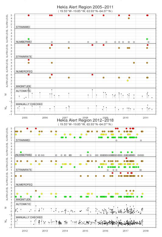
Figure 15. Temporal overview (2005–2018) of the numbers and types of alerts triggered based on the seismic activity at Hekla. The grey dots correspond to level 1, green to level 2, yellow to level 3, brown to level 4 and red to level 5.
