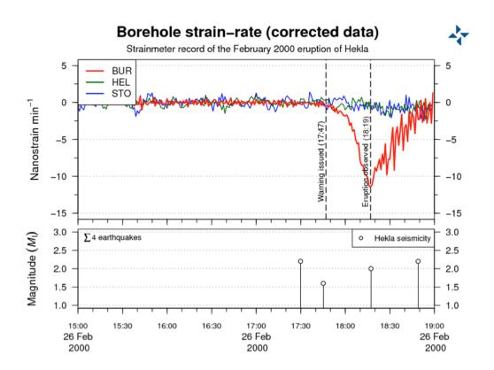
Figure 4. Strainmeter observations and earthquake activity prior to and during the 2000 eruption. The top panel shows the response of the strainmeters BUR (red line), HEL (green line) and STO (blue line). The bottom panel displays the earthquakes with M>1.5 detected prior to and during the eruption (data from IMO).
