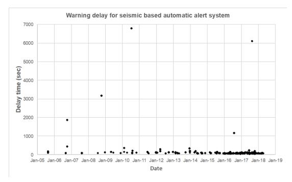
Figure 16. Warning delay time for seismic based automatic alert system.
