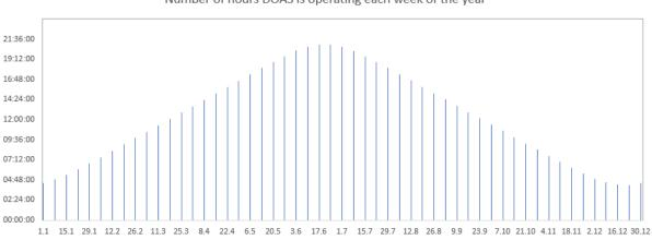
Figure 8. The number of hours for each day the DOAS can measure  $SO_2$  in the atmosphere for each week of the year based on sunrise and sunset times.
